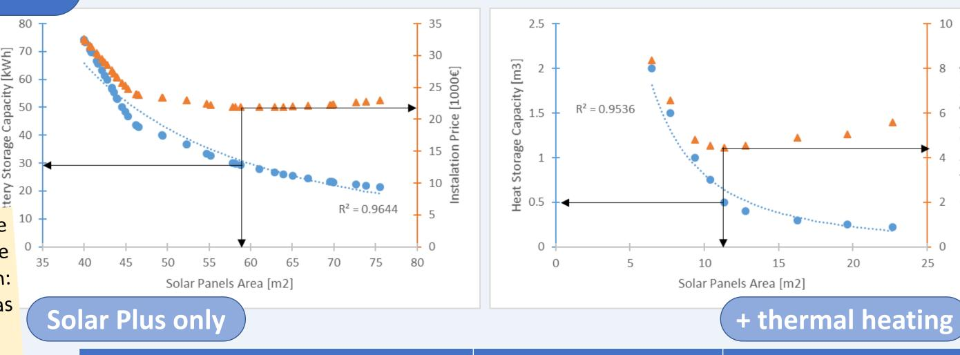
Solar Plus only + thermal heating PV + Solar Thermal Area  $59 \text{ m}^2$  $12 \text{ m}^2$  $0.5 \text{ m}^3$ Battery + Heat Storage 30 kWh Installation costs 4 200 € 22 000 € 0.08 €/kWh Levelized Cost of Energy (LCOE) 0.25-0.30 €/kWh
